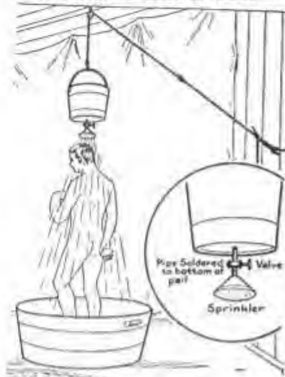
A Shower Bath That Costs Less Than One Dollar to Make
